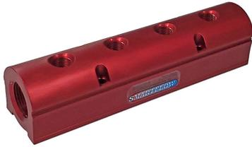
PCS offers Smartflow® Aluminum Water Manifolds to help optimize the mold cooling process along with reducing the amount of time to make a mold change to support SMED practices. The Aluminum Water Manifolds are made from proprietary extrusions cut to length, then machined and polished before the hard-coating anodizing process to color them red and blue. Utilize the red and blue color coding to denote supply & return cooling circuits.
