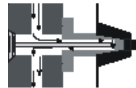
Conventional core cooling using a brass baffle.
