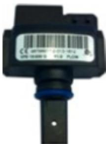
The *Smart Manifold* is equipped with very compact sensors that are capable of reading both flow rate & temperature. The sensor is based on the vortex flow measurement principal, which uses a bluff body in the middle of the flow path to create a small eddy current (vortices) and the pressure of this current is measured to determine the flow through a given cross sectional area.
