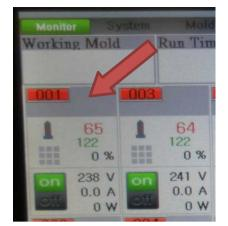
Below is the view of the individual zone set up page. On this page you will set up all the options to control this zone.
